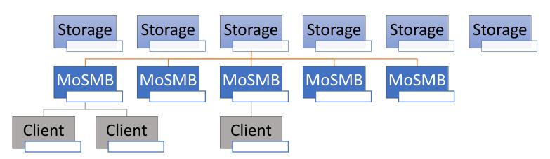
In order to produce high throughput and io parallelism from the system as a whole, one creates a set of servers who collectively serve out all the shares on the underlying storage. The underlying storage can be a clustered storage – clustered file system, object store
